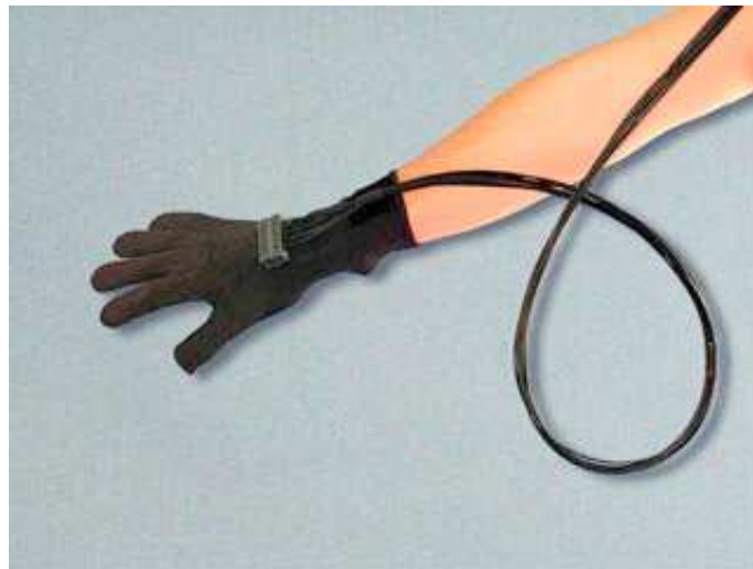
Figure 3.8: The 5DT Data Glove 5 MRI. This includes five sensors recording the relative degree of flexion/extension of each of the digits. These work via optical fibres: the increased attenuation of transmitted light brought about by mechanical deformation is used to determine how bent each finger is. The glove itself is made of Lycra, and the MR-incompatible control box remains in the scanner control room, with communication taking place over a 7m fibre-optic cable passed through the waveguide.
