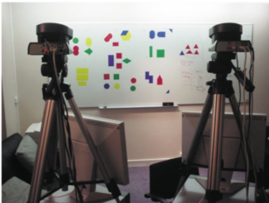
Figure 3.1: The setup for Luc Steels' Talking Heads experiment. One of the two embodied robotic agents is chosen as the speaker. The speaker randomly picks one of the coloured figures as the topic and transmits a word to communicate it to the hearer. The hearer has to guess the intended topic on the basis of the word used by the speaker. Figure taken from Steels (2003).
