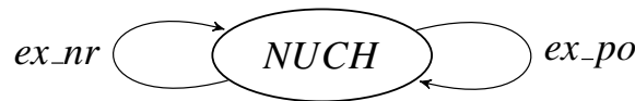
Figure 10.12: The behaviour of a macro-cell channel used for serving near users. The rate of the action ex\_nr is r_{ex\_nr} and the rate of ex\_po is r_{ex\_po} where r_{ex\_po} > r_{ex\_nr} .
