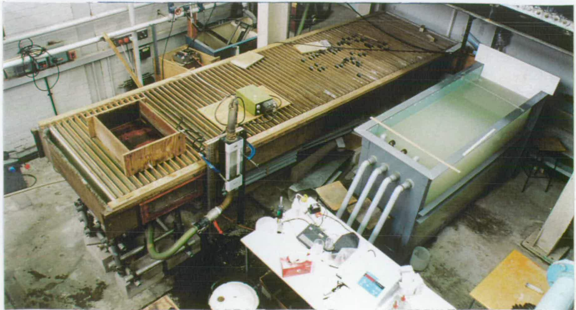
Figure 4.4.2 Channel flocculator in position
