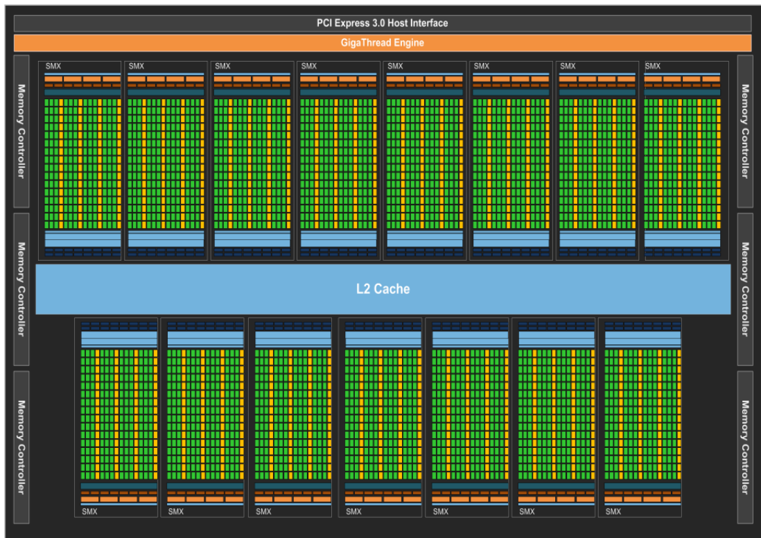
Figure 2.3: The NVIDIA Kepler GK110 architecture. From [NVID 14].
