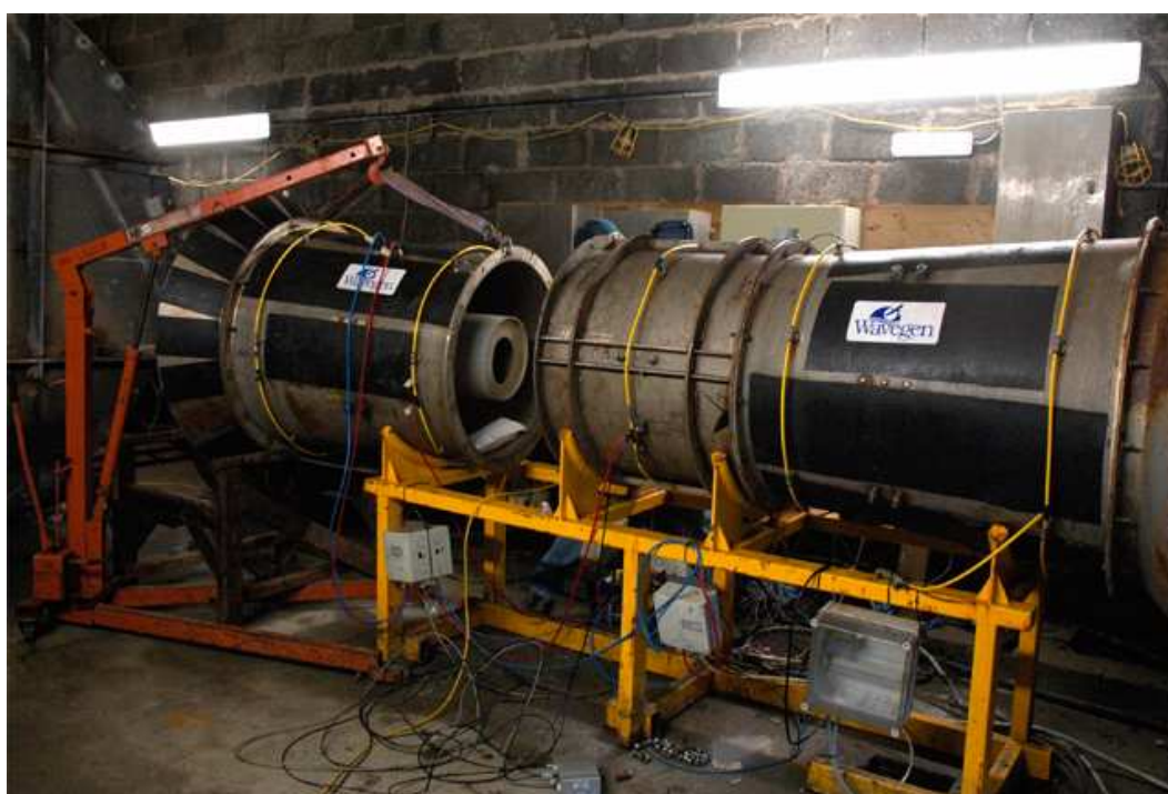
Figure 71: Steady state test rig ductwork separated for sensor installation
