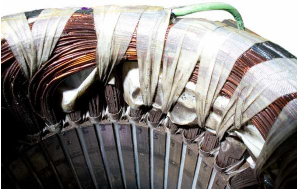
Figure 14: Endwinding and winding entering slots in an induction machine
