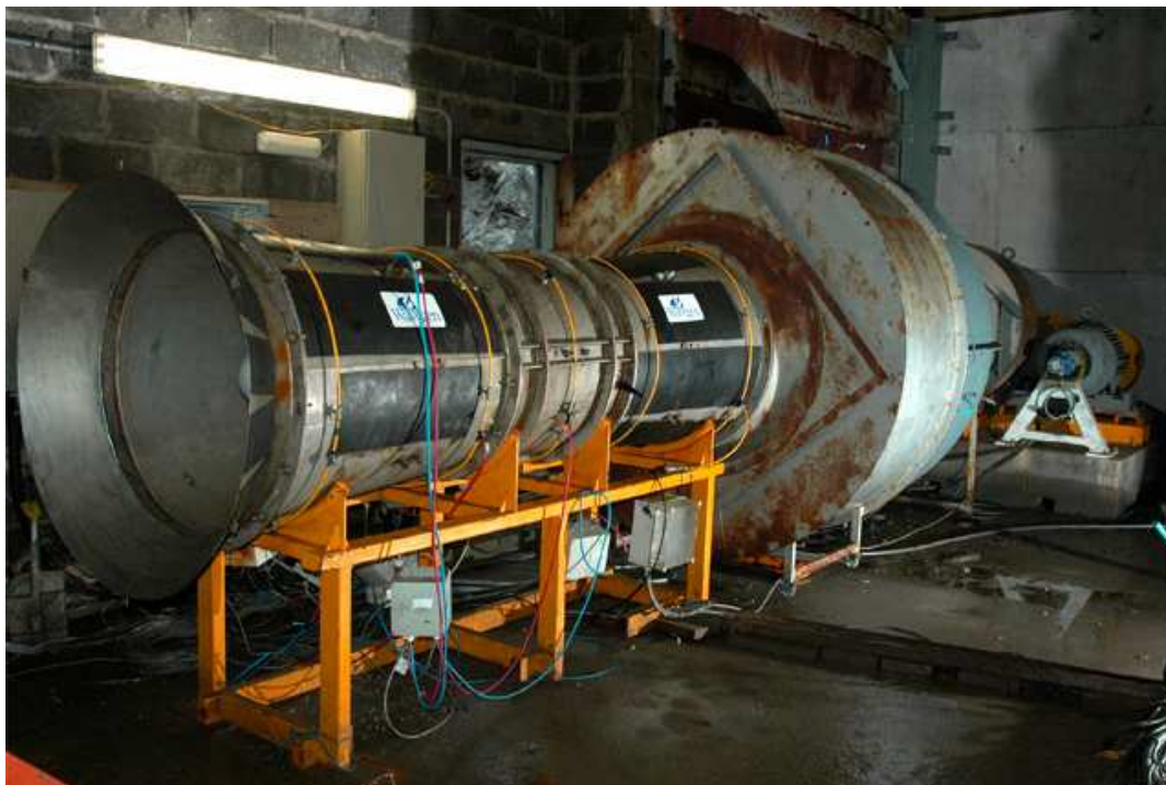
Figure 72: Test rig in LIMPET turbine hall. Turbine in foreground, settling chamber and fan motor in background
