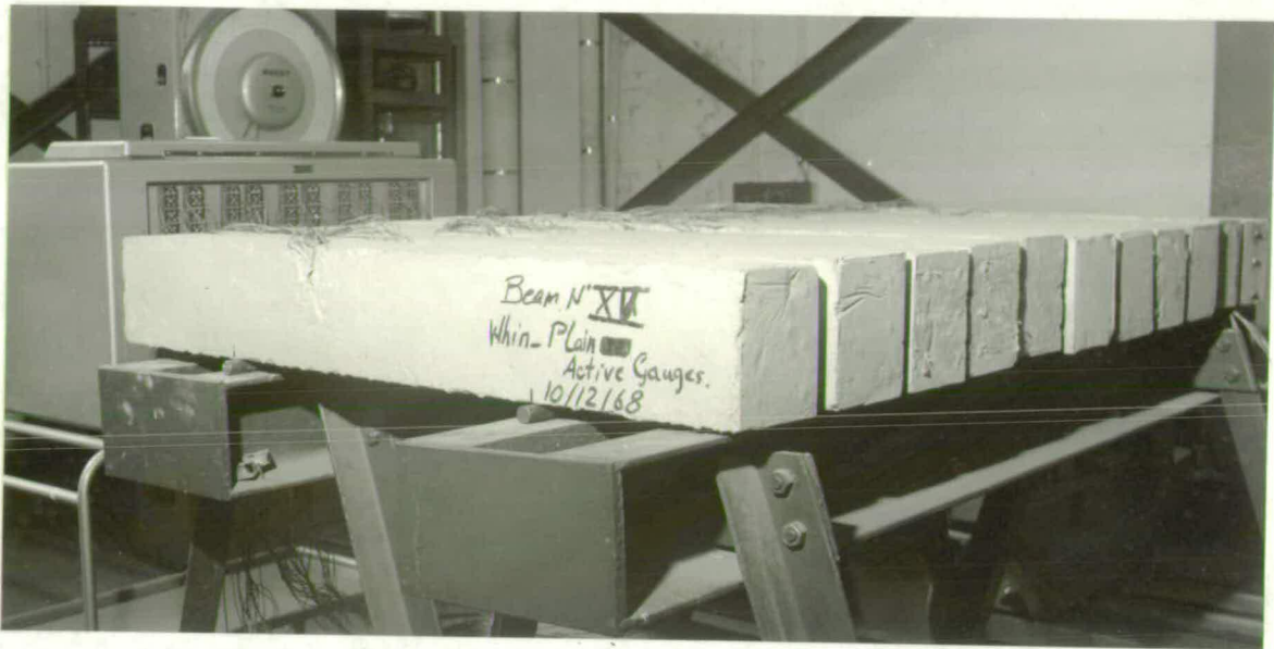
Plate 4.7 Beams under test for internal shrinkage strains.
