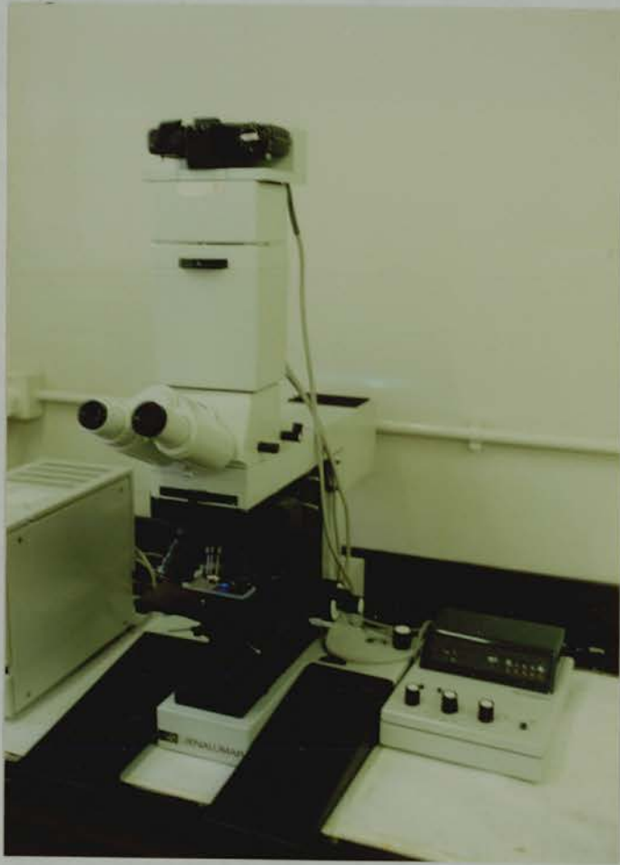
Figure II.4: A Carl Zeiss Jena optic microscope fitted with an automatic photomicrographic camera (mF AKS)
