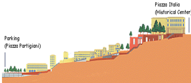
Figure 117. Perugia, Schematic section showing the system of escalators.
