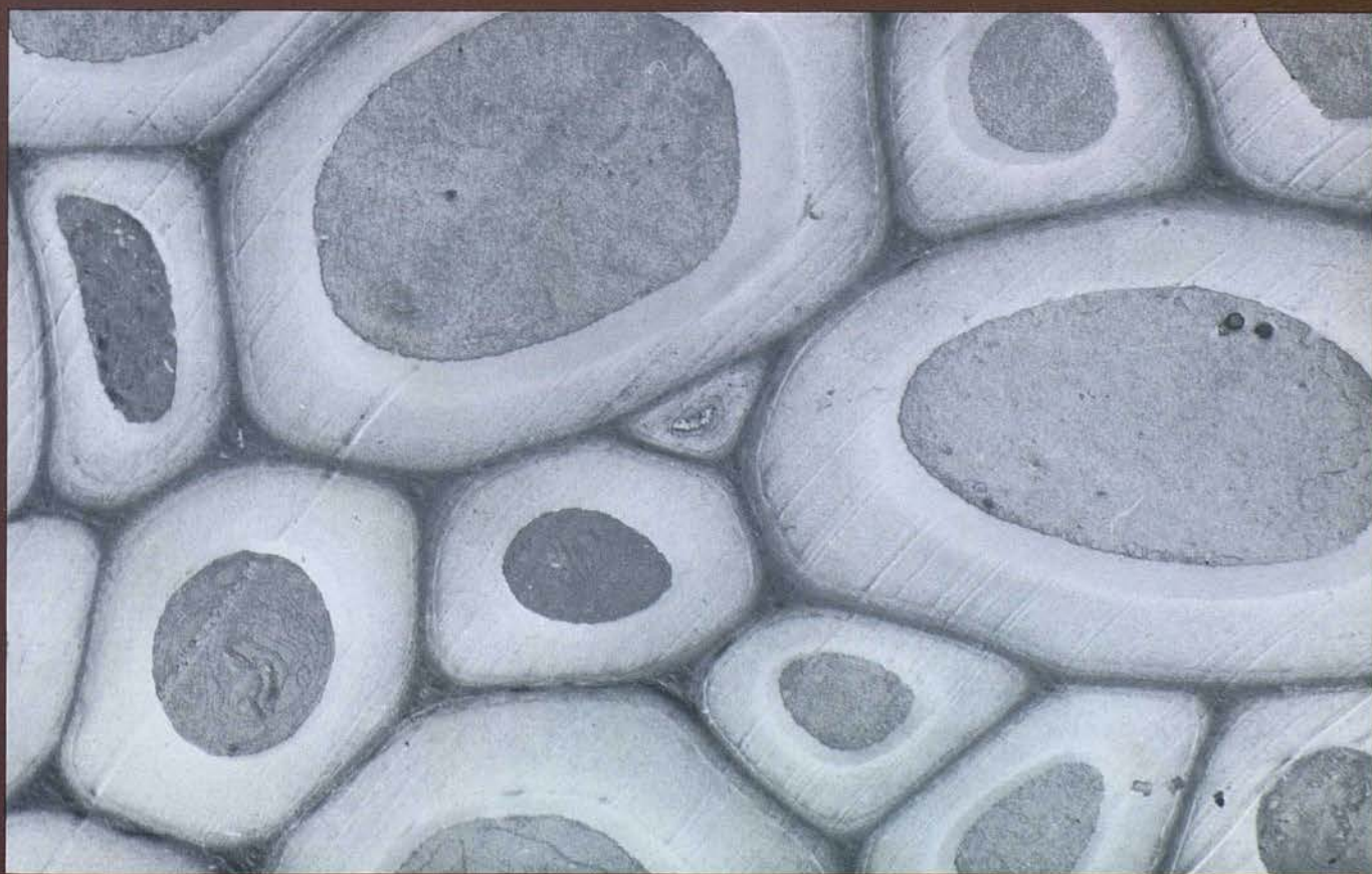
ELECTRON MICROGRAPH OF LOCUST WOOD ( ROBINIA PSEUDOACACIA ) (SOME KNIFE MARKS VISIBLE) MAGNIFICATION 7,700X
