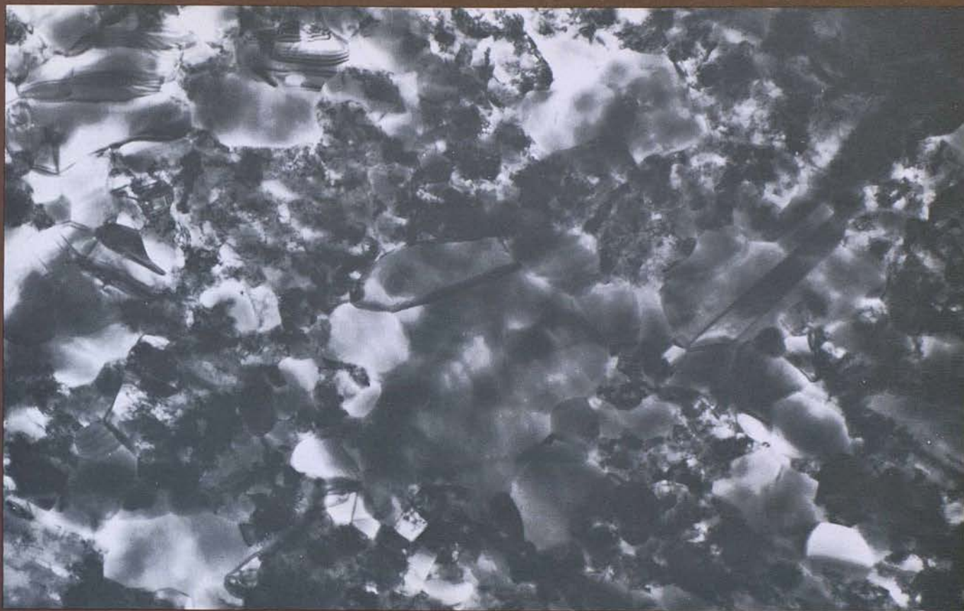
ELECTRON MICROGRAPH OF COPPER SECTIONED WITH A DIAMOND KNIFE. THICKNESS APPROXIMATELY 50 \mu MAGNIFICATION 30,000X
