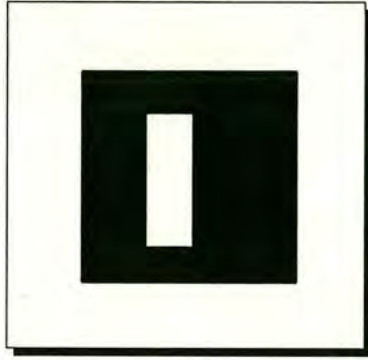
Fig. 1.3 Brown and Lohmann method. Firstly the hologram is sampled into evenly spaced square regions. Then the complex signal is represented in any square as a transparent rectangle with height proportional to amplitude and position proportional to phase.
