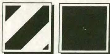
Fig. 2(a,b) missing pixel hologram and its FT.
