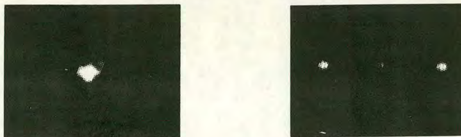
Figure 3: Diffraction from a simple grating (a) unplanarised EASLM, (b) planarised EASLM.
