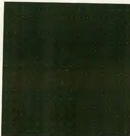
Fig. 1. Optical diffraction pattern from a Dammann grating.
