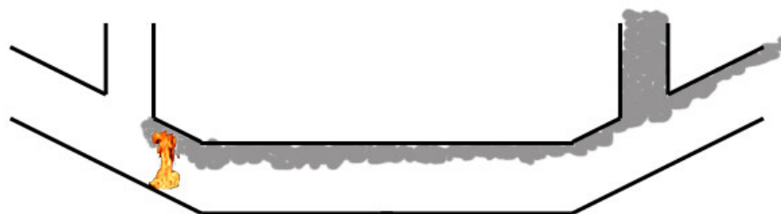
Figure 1: Schematic diagram of the hypothetical tunnel, depicting the worst case position for a fire (See Ch. 2.1)
