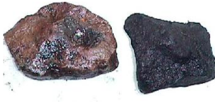
Figure 4: Detail of cleaned and contaminated rail ballast showing residual contamination
