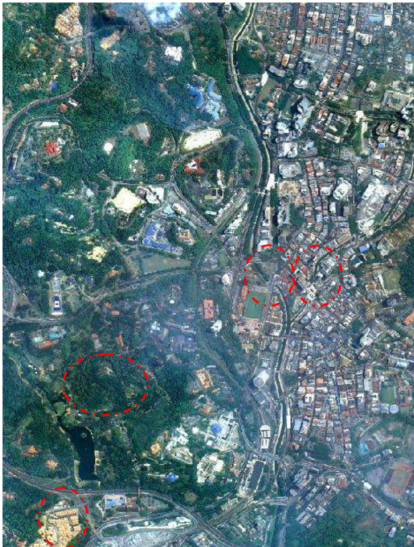
Figure 5.12: Image classification result for selected area in Zone 6 (Level Two – 40 scale parameter). Red circles labelled (a) and (b) illustrate some areas of misclassification
