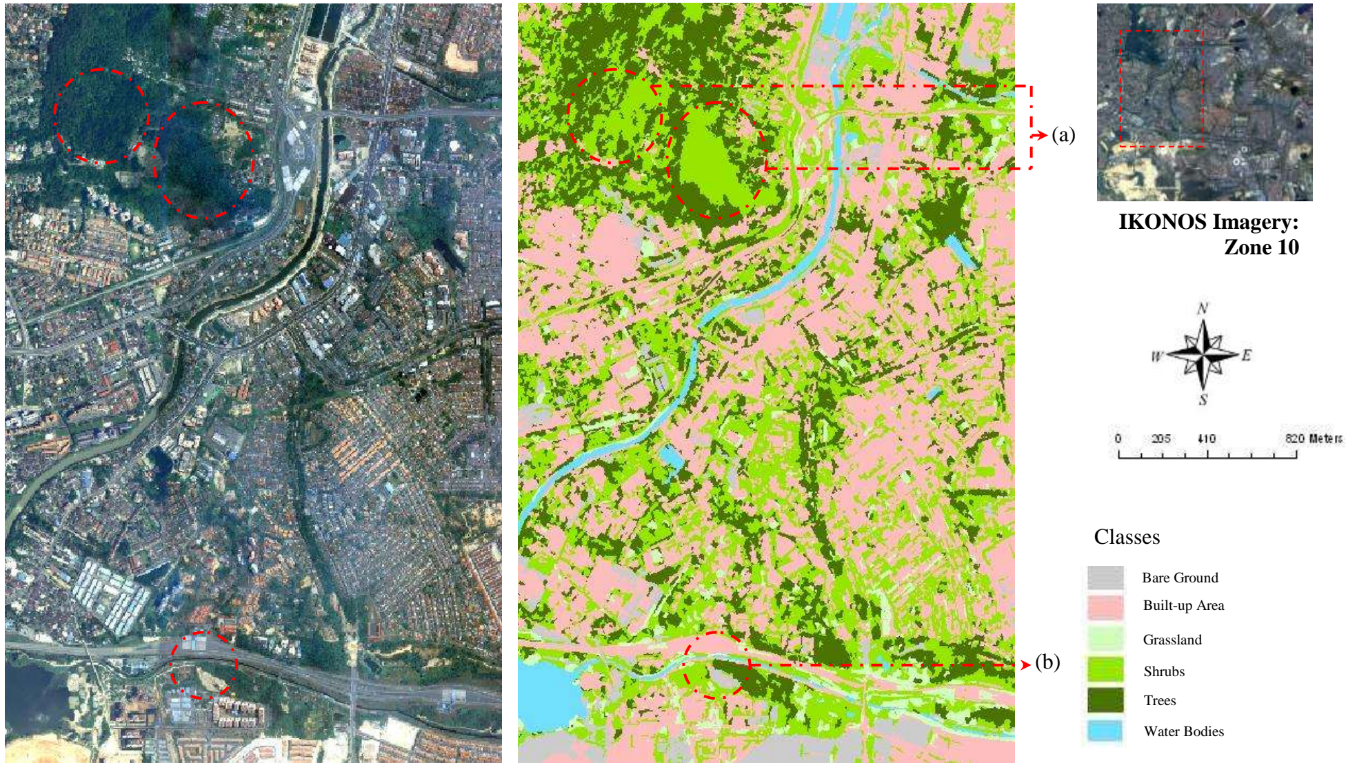
Figure 5.13: Image classification result for selected area in Zone 10 (Level Two – 40 scale parameter). Red circles labelled (a) and (b) exemplify areas of misclassification.
