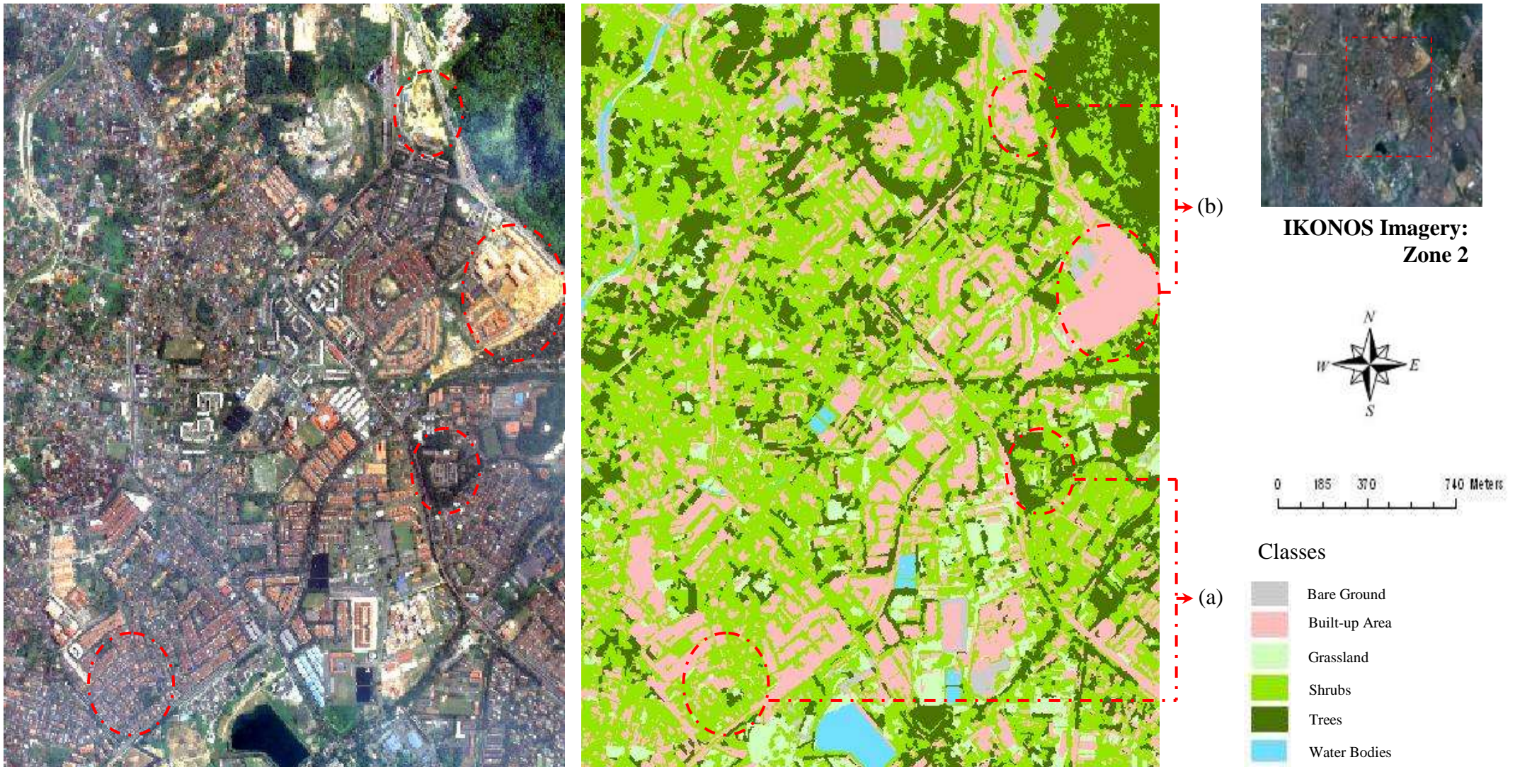
Figure 5.11: Image classification result for selected area in Zone 2 (Level Two – 40 scale parameter). Red circles labelled (a) and (b) illustrate some areas of misclassification.
