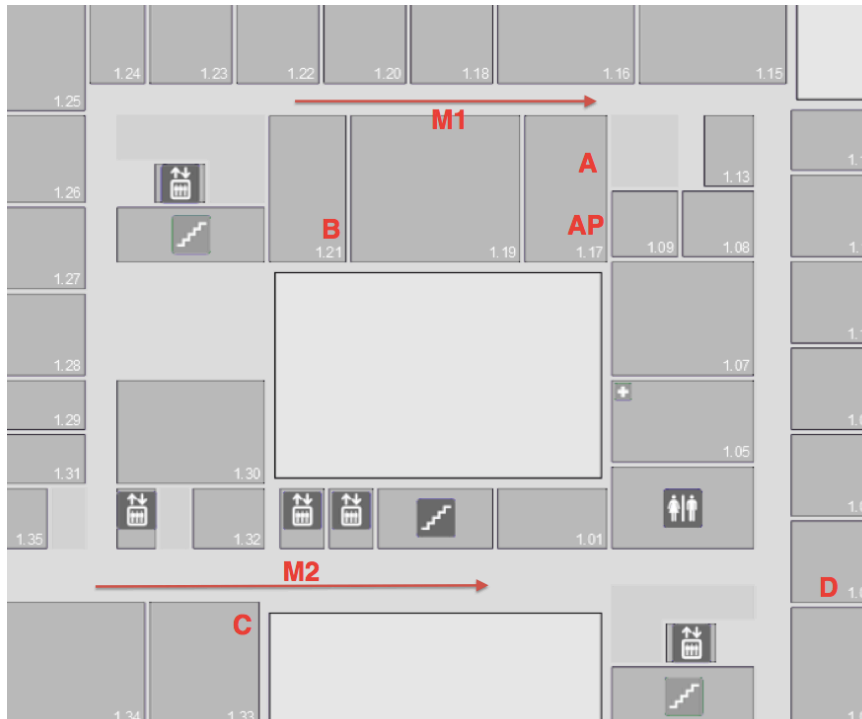
Figure 5.1: A snapshot of the 802.11n WLAN testbed layout on the floor map.
