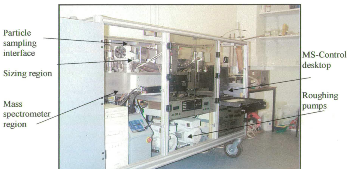
Figure 2.1. A photograph of the ATOFMS (TSI 3800)
