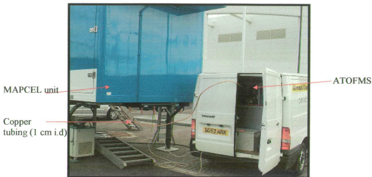
Figure 6.3. A photograph of the ATOFMS instrument sampling from the upstream/downstream air flows of the MAPCEL-VACES unit.
