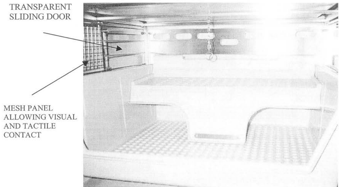
Plate 5.1 Interconnecting rabbits cages, showing the transparent door which can be opened to allow rabbits access between two cages and the mesh panel that allows visual and minimal tactile contact between rabbits
