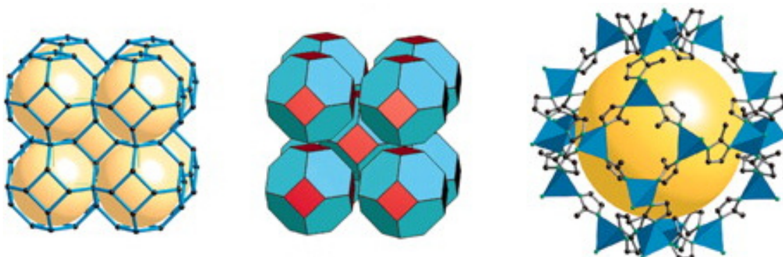
Figure 2.9 The single crystal x-ray structures of ZIFs. (left and center), the net is shown as a stick diagram (left) and as a tiling (center). (right)The largest cage in each ZIF is shown with ZnN 4 tetrahedra in blue, H atoms are omitted for clarity [56].
