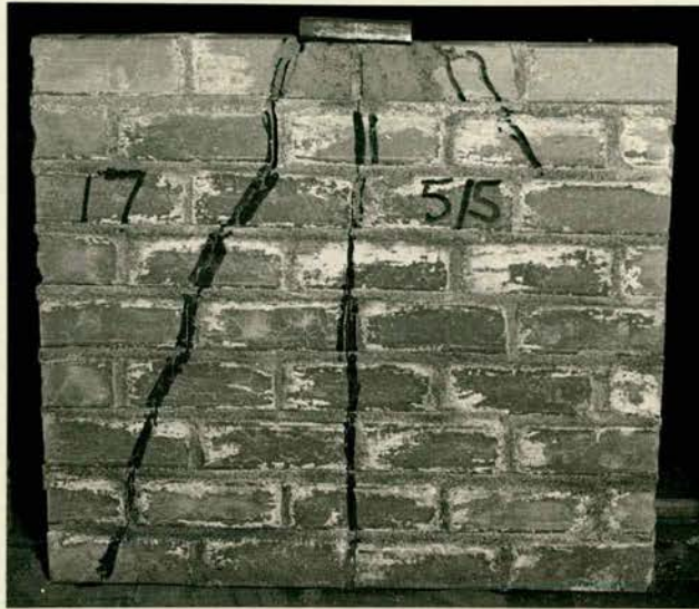
1/3rd. Scale Brick Wall - Central Bearing Plate - Failure by Vertical Cracking, Local Spalling, and Diagonal Shear Crack.
