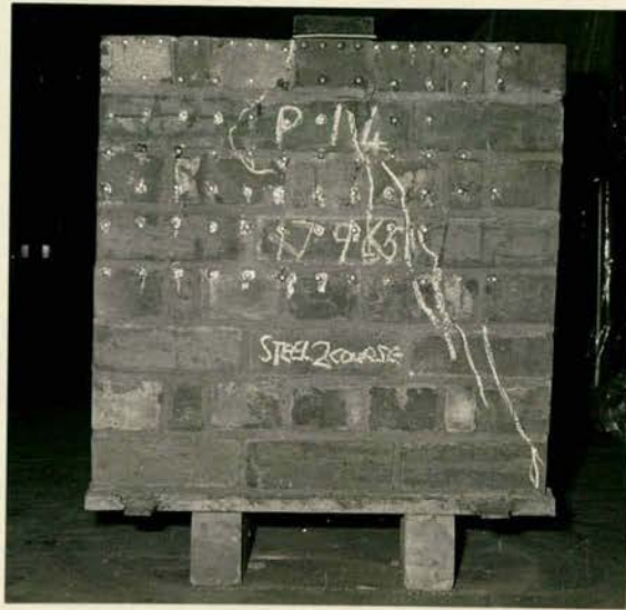
A Typical Wall, No. 14 - Showing Demec Studs for Strain Measurements, and Failure Mode. Plate 3-5
