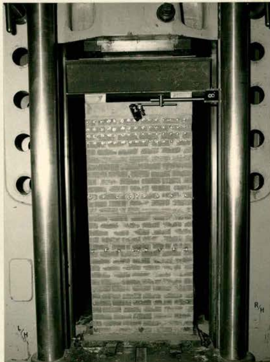
1/3rd. Scale Cavity Wall in Testing Machine Demec Stud Positions.
