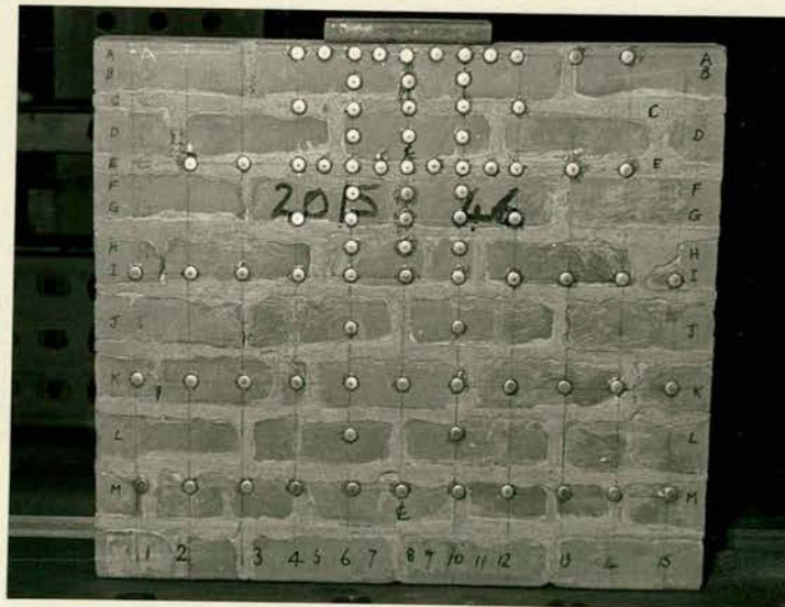
1/3rd. Scale Brick Wall - Demec Stud Positions for Central Bearing Strain Measurements.
