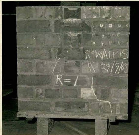
A Typical Failure - 4\frac{1}{2} " Central Bearing Plate. Plate 3-3
