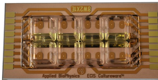
Figure 3.2: ECIS Medusa array. A picture of an ECIS Medusa array. Each well has two 250 \mu\text{m} diameter working electrodes. Only four wells can be connected at a time [332].
