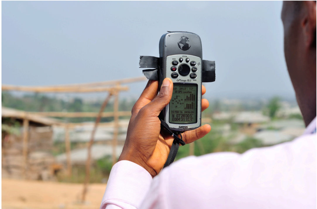
Figure 47 Taped handheld GPS receiver (Garmin GPSMAP 76S) during student training in Ile-Ife (Thorpe 2016).
