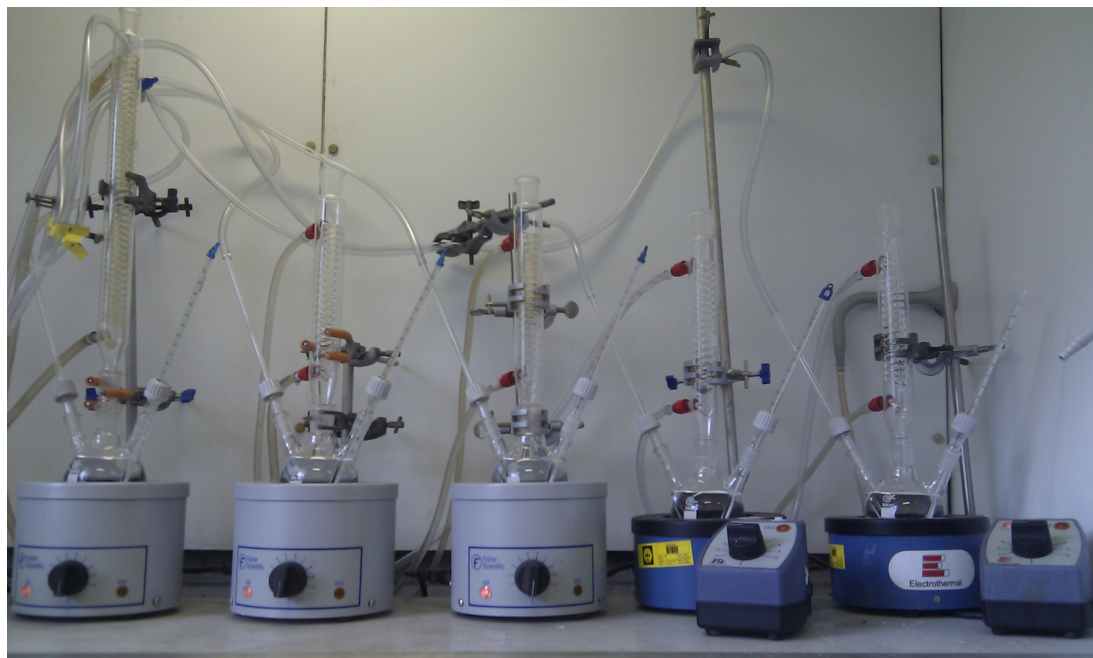
Figure A.1: CO 2 batch experimental setup, comprising (left-to-right) flasks F1 - F5 set on heating mantles set to 58°C, each with glass condensing coil, thermometer, glass CO 2 feed rod and rubber CO 2 feed tubing from a vapour withdrawal CO 2 bottle.
