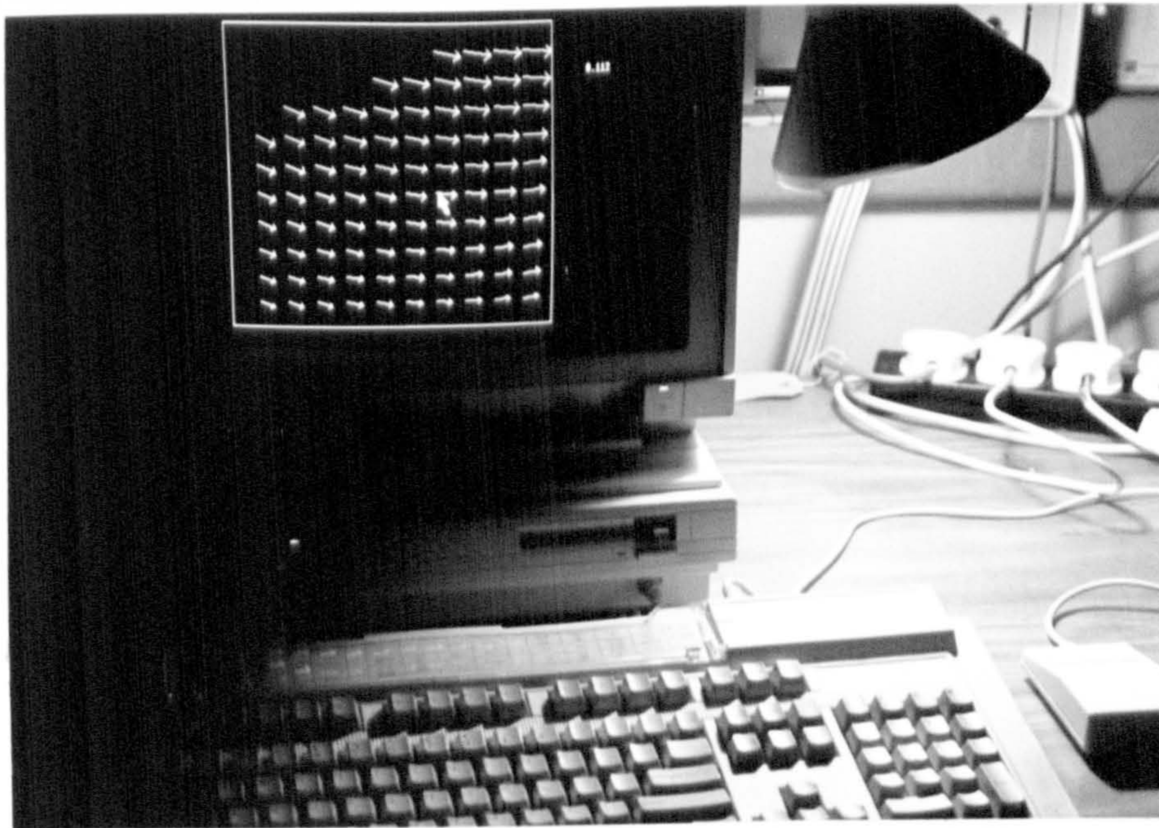
Figure 5.2: The interactive editing program allows the velocity data from the analysis of PIV negatives to be viewed and assessed visually. Magnification of smaller areas, removal of spurious vectors and interpolation are performed via the mouse, permitting rapid and precise processing of small data sets.
