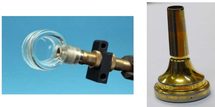
Figure 3.11: At left is the transparent mouthpiece developed by Richards[Richards, 2003]. Also shown is the mouthpiece support mechanism, attached to the mouthpiece from the right hand side of the photo. At right is a Dennis Wick 6BS trombone mouthpiece.
