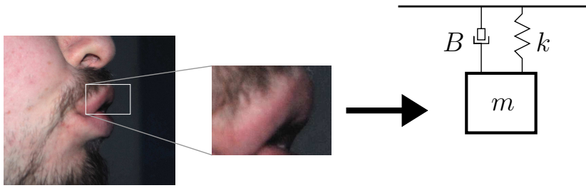
Figure 2.2: The macro-scale lumped element approach to musical valve modelling. The entire lip mass is condensed into a single ‘lump’ of mass m , connected to a rigid bounding wall with a spring of stiffness k and damping B .
