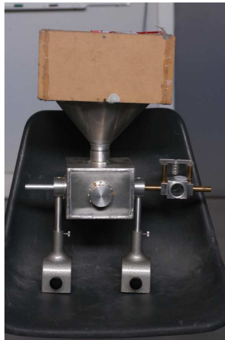
Figure 3.22: A photograph showing the acoustical driving system used for the human lip mechanical response measurements. The loudspeaker is contained in the wooden box and a reverse cone connects it to the main coupling cavity which is filled with acoustical damping foam. On the right hand side of the box is a hole available for connection to a mouthpiece.
