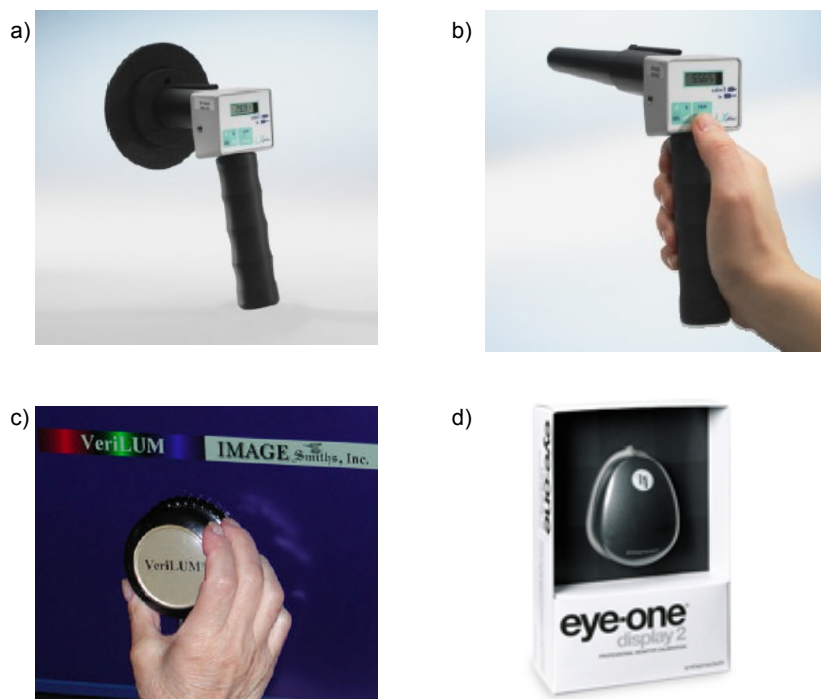
Figure 5.11. – Photographs of different photometers. a) IBA LXPlus in contact mode; b) IBA LXPlus in telescopic mode; c) Image-Smiths' VeriLUM contact pod; d) X-Rite eye-one Display2 contact pod.
