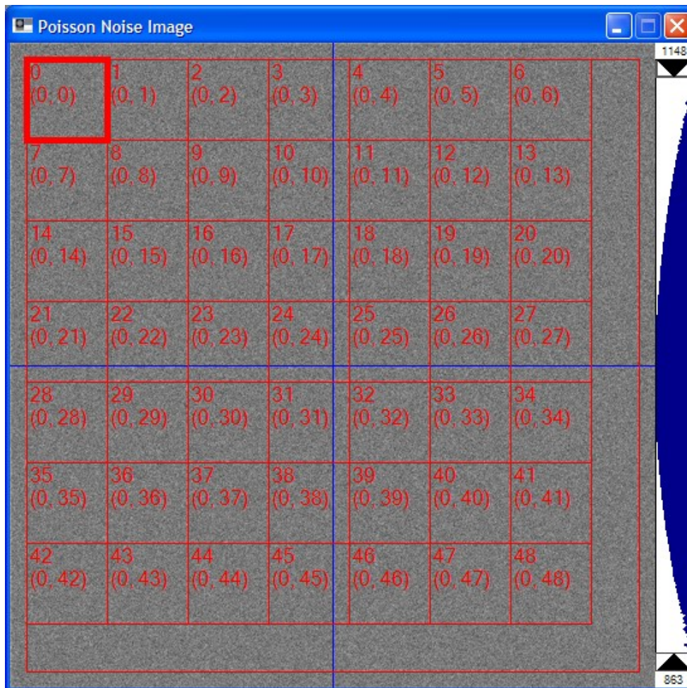
Figure B.14. – Screenshot of the noise image generated by IQWorks to validate the Noise Power Spectrum (NPS) calculation algorithms. Details of the parameters used to generate the image are included in the main text. Regions of interest (ROIs) automatically placed for the analysis are indicated by the red squares, each of which is referenced by a unique number (a, b) where a is the layer number and b is the index of the ROI in the layer. In this example the first layer of a 10 layer image is displayed, so a = 0 . The bold red square at the top left is the ‘reference ROI’ against which the results in all other ROIs are normalised.
