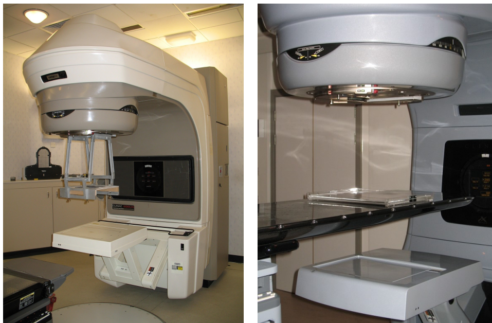
Figure 3.25. – Options for aligning the QEPI1 phantom at isocentre. Left–The phantom is mounted on an assembly attached to the linac gantry. Right–The phantom is embedded in a PMMA jig which is positioned on the treatment couch.
