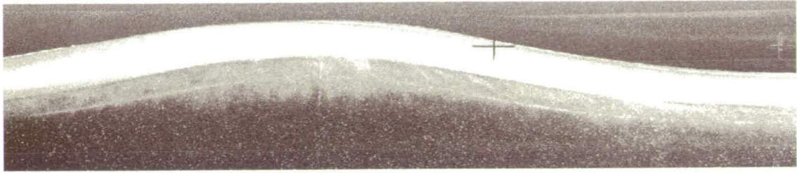
Figure 4.22: Upper section of a DPIV image taken at t=7.23s following paddle initiation. Notice the laser light reflections (broad band of white light) and the pollen in the free surface region (greyish patches).
