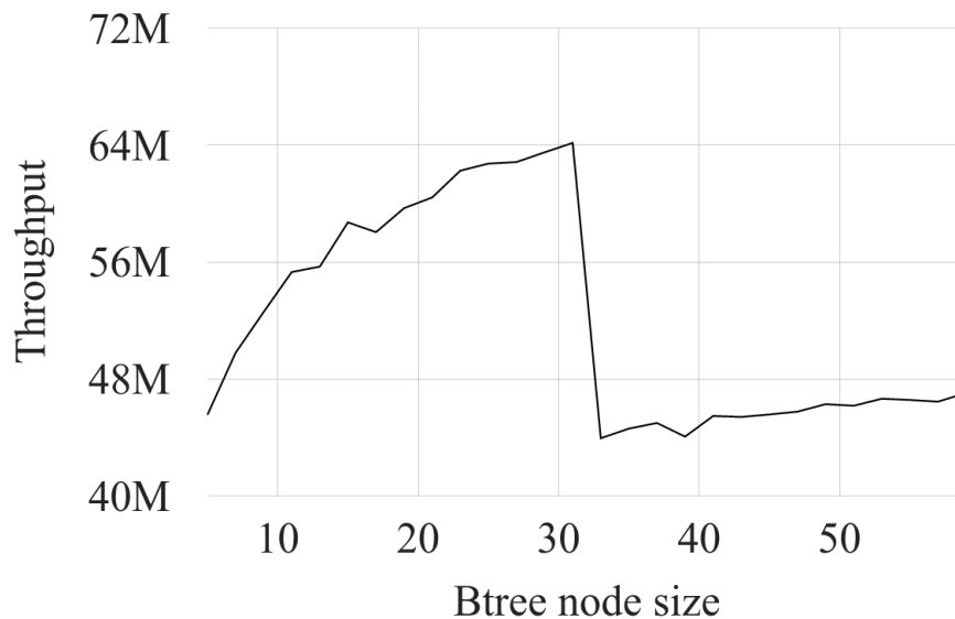
Figure 4.10: Effect of BTree node size on throughput ( n -gram queries per second)
