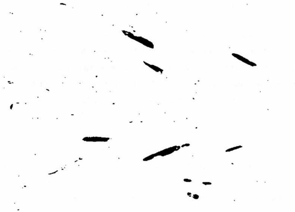
Figure 4.3: Boolean AND image derived from thresholding in the green and blue channels of the RGB image
