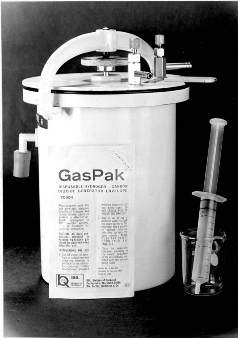
FIGURE 8. - The Gaspak envelope and the BTL anaerobic jar. The side arm of the jar is sealed.
