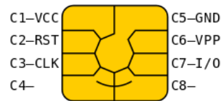
Figure 2.1: The contacts of a smart-card: VCC is the power, RST is the reset, CLK is the clock signal, GND is the ground connector, VPP is the programming voltage and I/O is the input/output connector.
