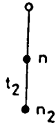
Figure 4.22 A single-site hopping diagram representing an unpaired anion hop from the site n onto the site n_2 .
