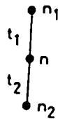
Figure 4.19 The single-site hopping diagram for the site n . The diagram represents an anion hopping from site n_1 to site n at time t_1 with another anion hopping from site n to site n_2 at time t_2 .
