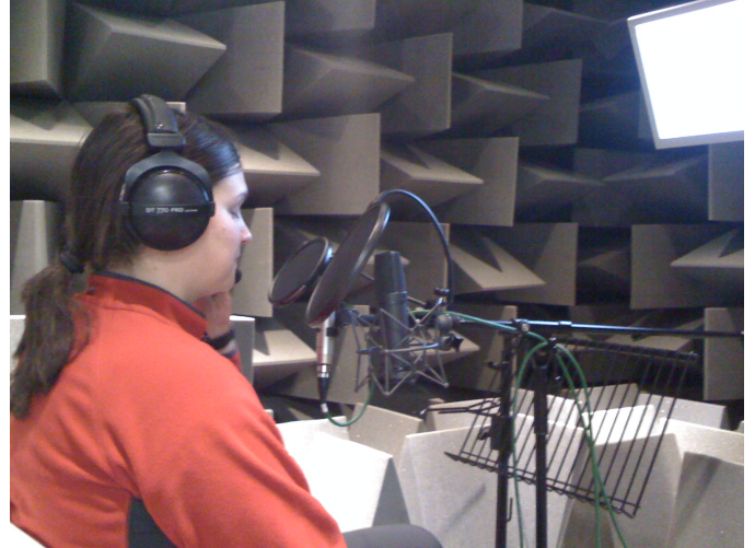
Figure 1: Studio setup for recordings. Left microphone is a Sennheiser MKH 800 and the right one is a Neumann u89i. The headset has a DPA 4035 microphone mounted on it.
