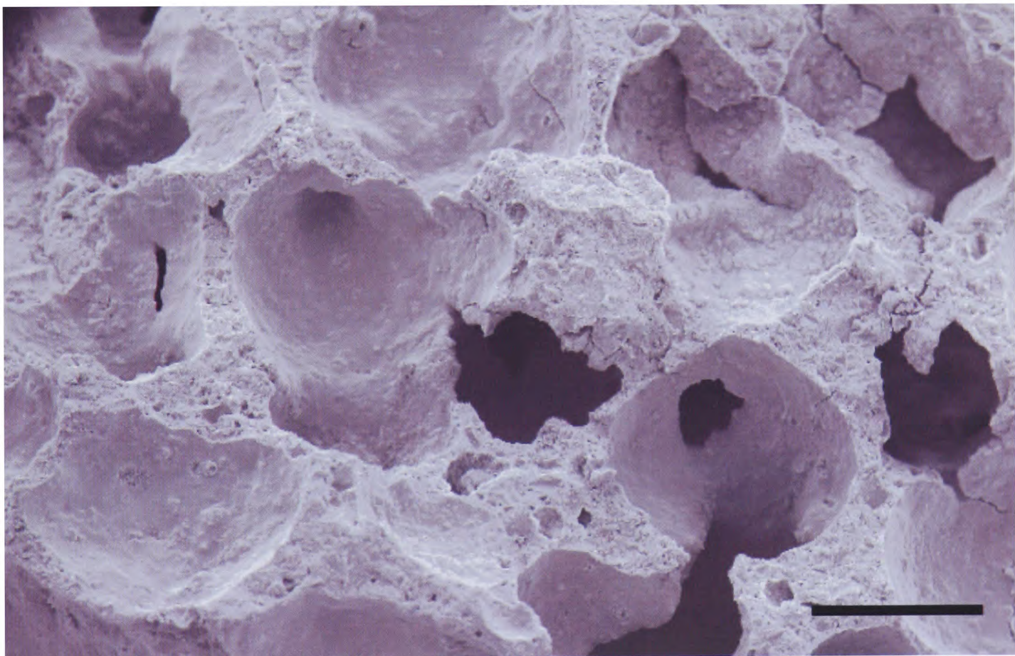
Figure 6.3: Low magnification SEM image of AAC microstructure: aeration pores. Scale bar represents 500 \mu\text{m} .
