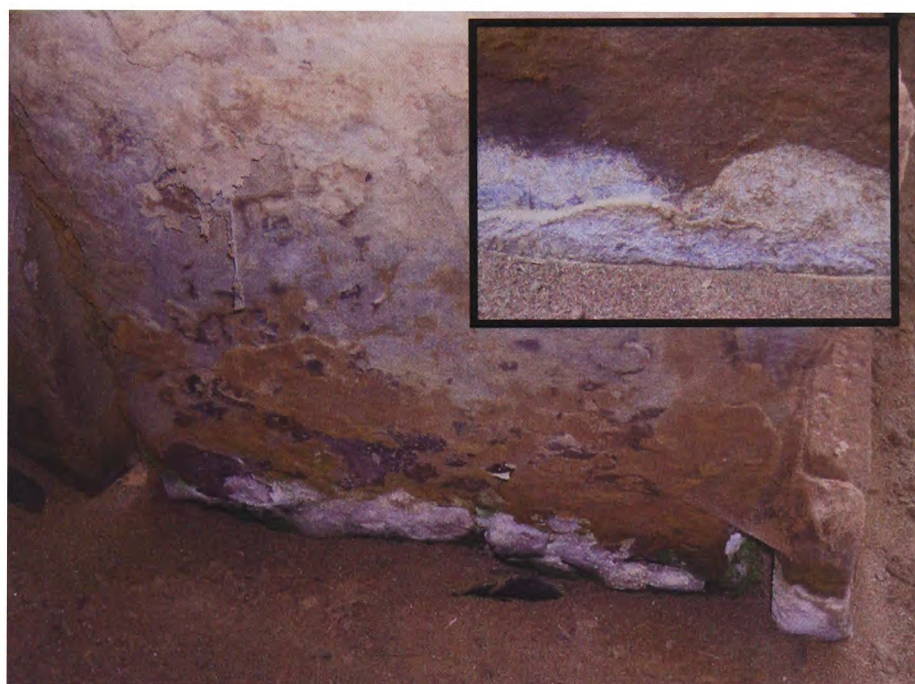
Figure 5.8: Salt lines on the same stone as figure 5.6, but taken in Aug/Sept 2004. Small corner image is a higher magnification view of the salt. Scale indicated in caption for figure 5.6.
