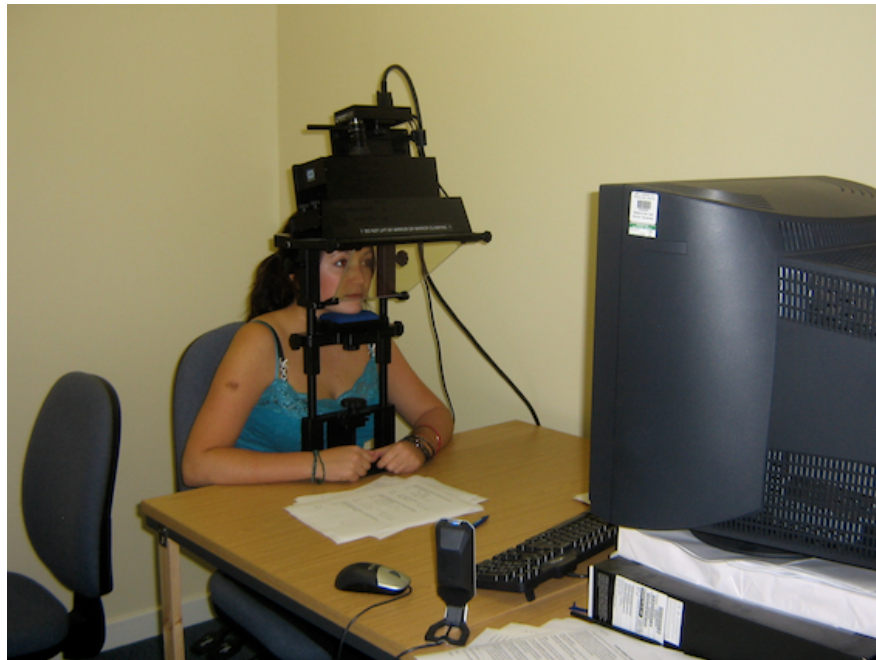
Figure 2.1: Eye-tracker used for the experiment presented in this chapter. With this type of eye-tracker, the head of the participant is fixed using a chin and forehead rest. The position of the eyes is measured using an infra-red camera and light, through the semi-reflective glass in front of the participant's face.
