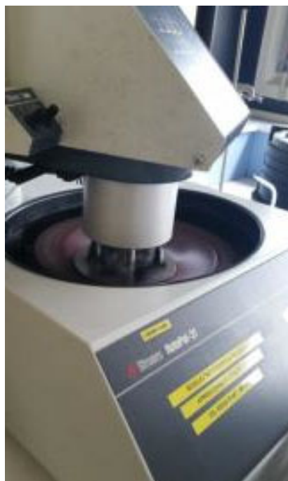
Figure 7.6: The last step in the polishing process involves repeating step 3d) to remove any excess diamond product.
