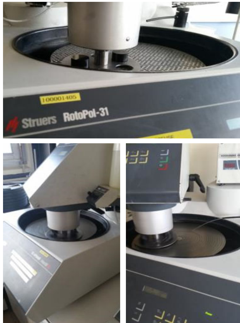
Figure 7.3: Polishing of the 2 samples. The bottom right image shows the use of lubricant during the polishing.
