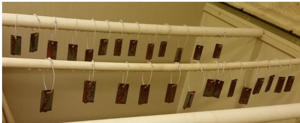
Figure 3.12: Coupons 25 to 46 immediately following 48 hours of salt spray treatment.
