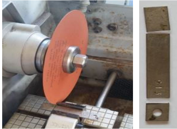
Figure 7.1 The slicing of coupon 913 into 2 small segments (right)
