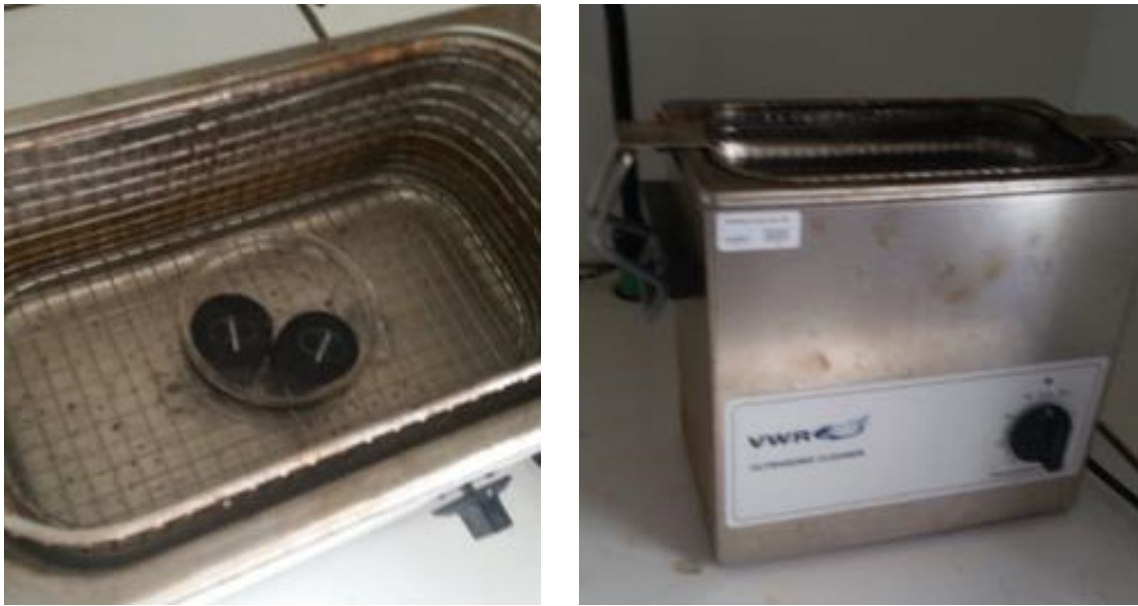
Figure 7.5: Specimens are agitated in an ultra-sonic cleaner to remove any excess lubricant.
