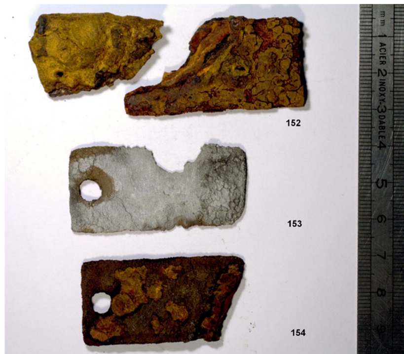
Figure 3.5: Appearance of corrosion coupons following 18 months of experimental tidal conditions
