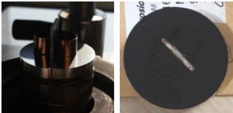
Figure 7.2: A coupon segment is held in place (left) and then set in epoxy resin with sliced area exposed (right)
