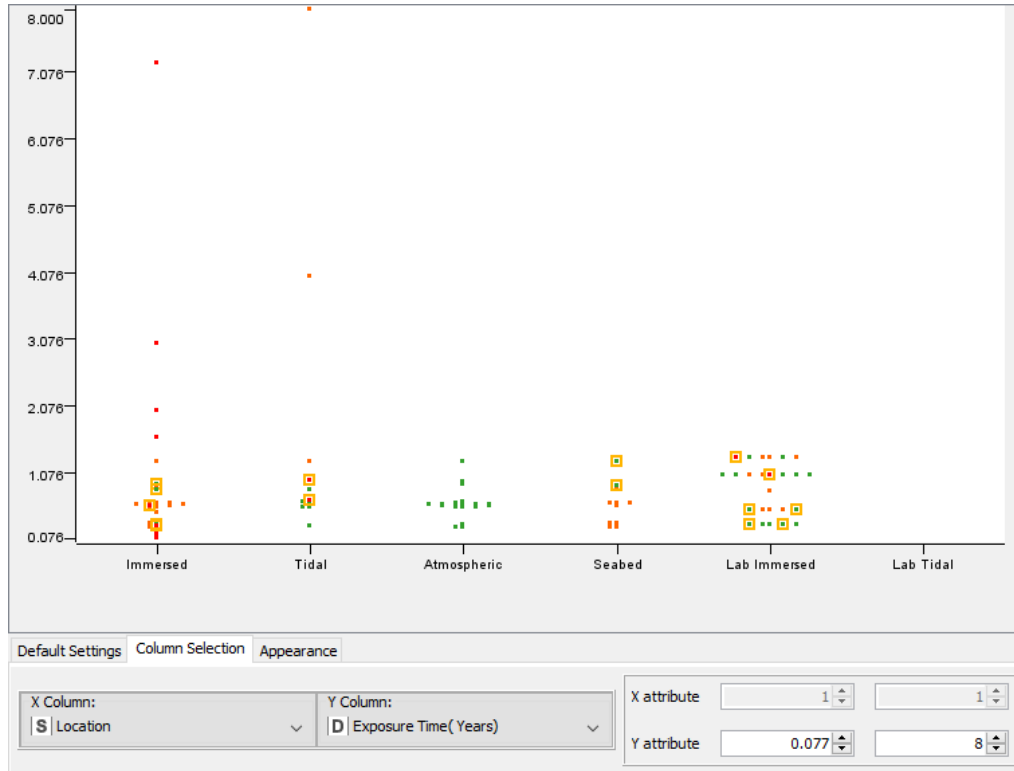
Figure 5.6: Predicted corrosion rates at each Location using decision tree model.
