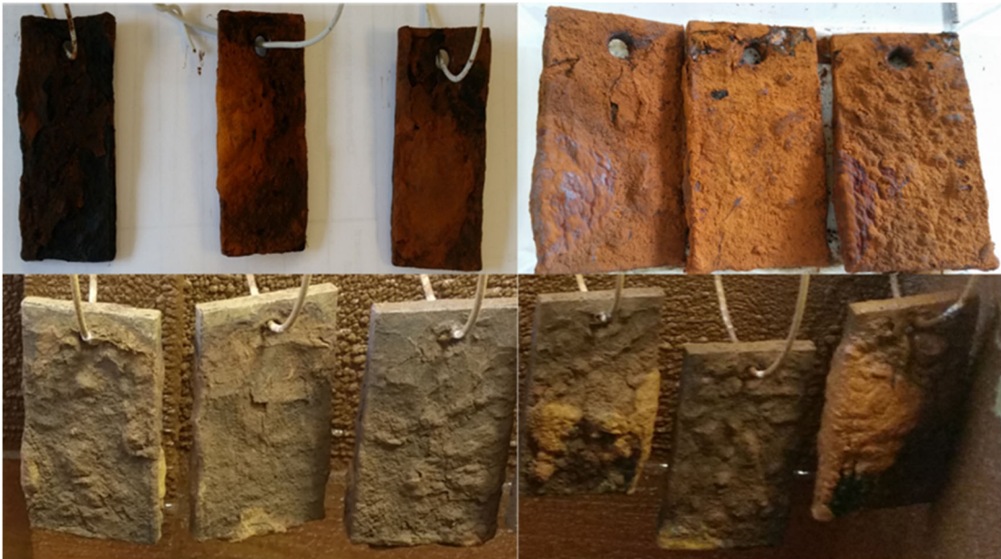
Figure 3.4: The accumulation of corrosion product on coupons extracted from the tidal chamber. From top left to bottom right the coupon exposure time was 3; 6; 9 and 12 months.
