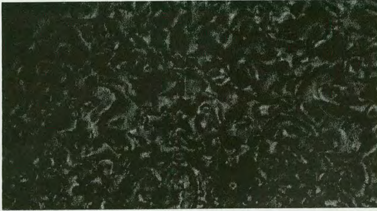
Figure 3.6: Microscope image of the pure nematic phase of 8CB under crossed polarisers. The disclination lines are predominately visible throughout the structure
