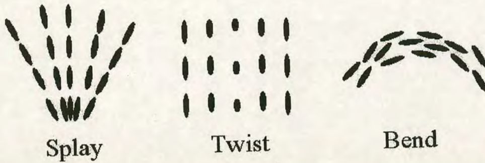
Figure 2.8: The three types of deformation in a nematic. Note that for twist the director rotates in out of the plane of the page
