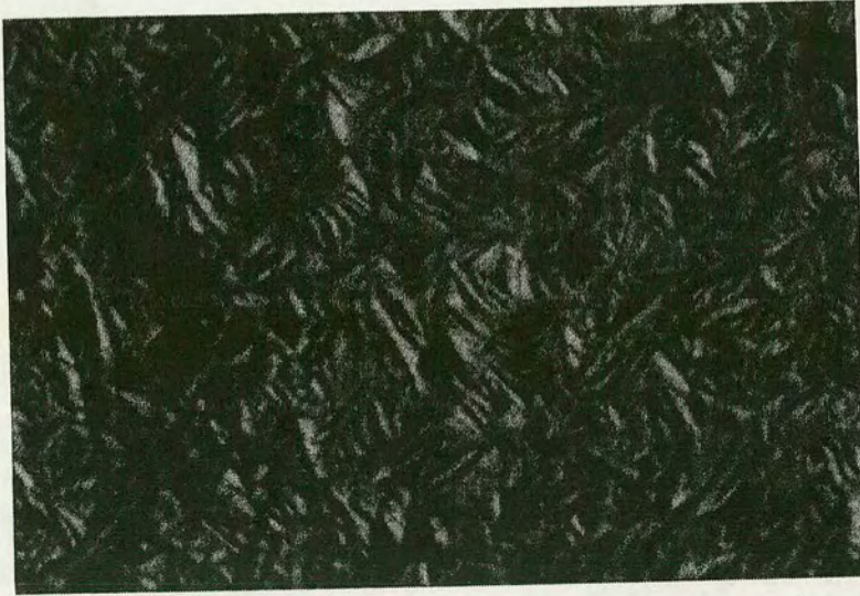
Figure 3.7: Microscope image of the smectic phase of 8CB. The fan regions are easily evident and small regions where the molecules have aligned homeotropically can also be seen as blank patches.
