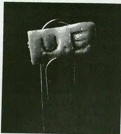
Figure 7.1: A slice of colloid liquid crystal composite. This particular sample was made from with a particle volume fraction of 20%, and at room temperature is so rigid that it can be cut with a knife. Picture courtesy of S. Meeker.
