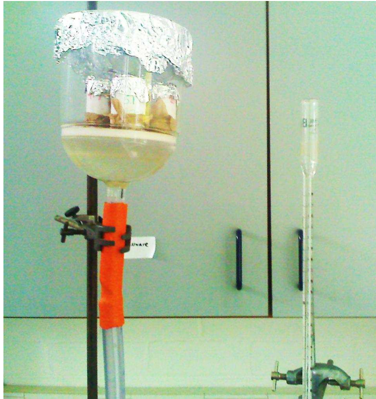
Figure 7.3: Tension plate apparatus
