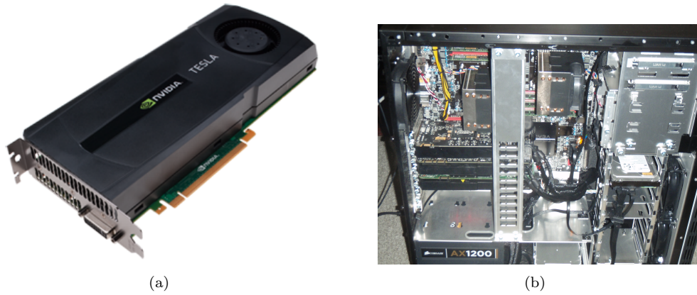
Figure 2.7: (a) A single Nvidia Tesla GPU aimed at the HPC market. (b) A single workstation housing 3 GPUs and 2 CPUs. Although of similar compute power, this configuration with 3 GPU in one machine is visibly less complex than the cluster shown in 2.5
