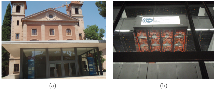
Figure 2.1: (a) The former church holding Mare Nostrum and (b) the row of racks inside the church showing the rack mounted servers and inter-connect. Even the simple concept of Mare Nostrum requires the complex, high speed backbone (the orange mass of cables, shown in the centre of (b)) to be fully exploited.
