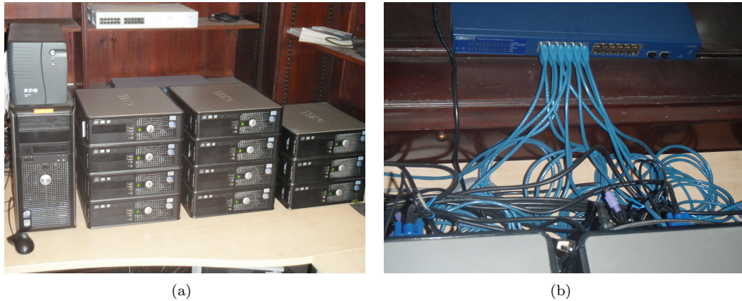
Figure 2.5: The small cluster bought in 2010 for the use of the Camp group in Edinburgh. The cluster consists of 11 quad-core compute nodes, connected by a fast ethernet router to a head node housing 2TB of storage. and Even a small cluster such as this requires a significantly complex backbone in order to be interconnected sufficiently as shown in (b).
