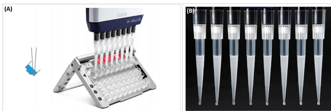
Figure 2-23. Transfer of GEMs for RvT incubation. (A) Aspiration of GEMs from recovery wells. (B) Opacity is indicative of a successful Chromium™ Controller run (adapted from manufacturer’s instructions, 10x Genomics, USA).
