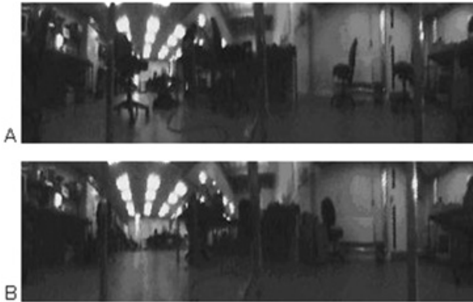
Figure 15 The moved landmarks experiment. A: The unfolded home image. B: An unfolded image taken from the home position after the changes in the scene.
