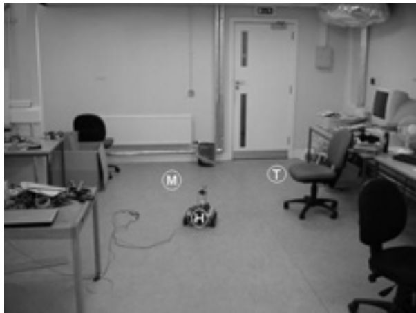
Figure 16 The moved chairs scene. H: The home position. M: The local minimum. T: The perceived home position for image warping.
