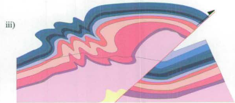
Figure 3.5: Two localities in Transect A have ambiguous fault geometries, a) is in the centre of the transect and b) at the south coast (see Transect A for locations). i) Map data, ii) south dipping normal fault, iii) north dipping reverse fault. In both instances the south dipping normal fault model is preferred, see text for discussion.
