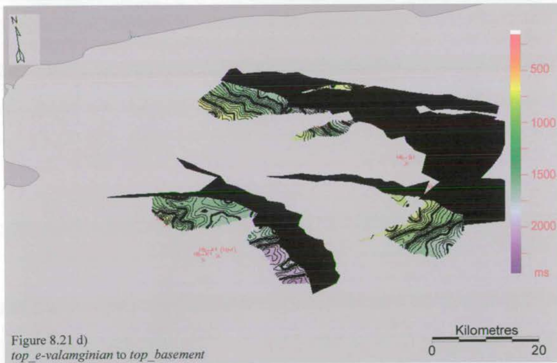
Figure 8.21: Cumulative isochron plots of thickness from top_basement to Principal Syn-Rift horizons: a) top_kimmeridgian , b) top_portlandian , c) top_berriasian , and d) top_e-valanginian . The calculated isochrons have only been plotted where the complete sequence thickness is present, resulting in the decrease in areal extent from (a) to (d). As the extent of top_l-valanginian is very restricted it has not been plotted.
