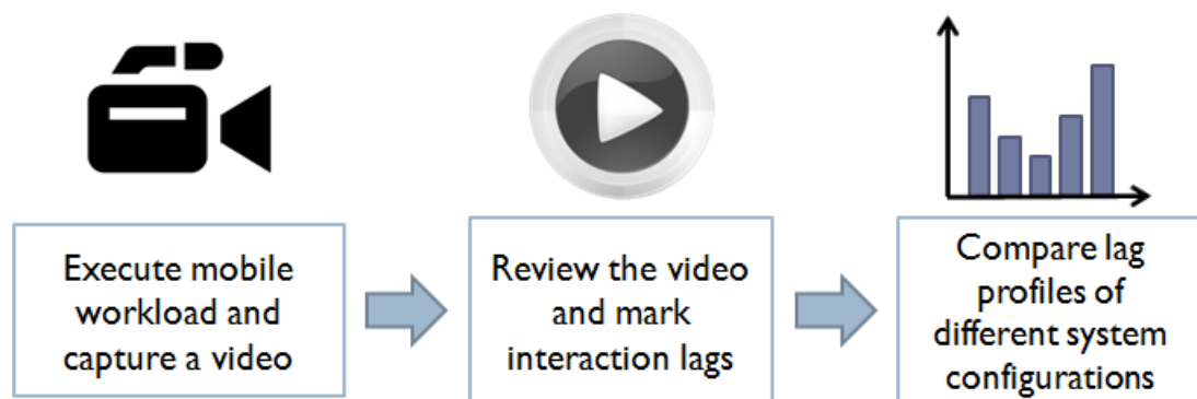
Figure 4.1: Execute an interactive workload and record screen output in a video. Automatically identify interaction lag timings in the video and evaluate them in terms of user satisfaction.
