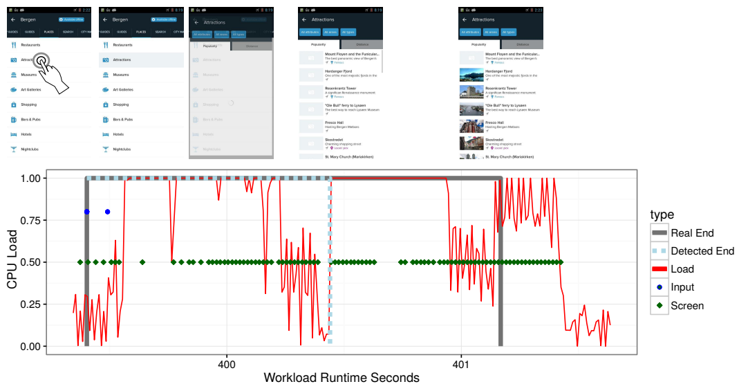
Figure 6.14: Sample workload of an early lag end detection. Low load and a pause after a screen burst lead to a false positive ending report by the heuristic in the middle of the lag.
