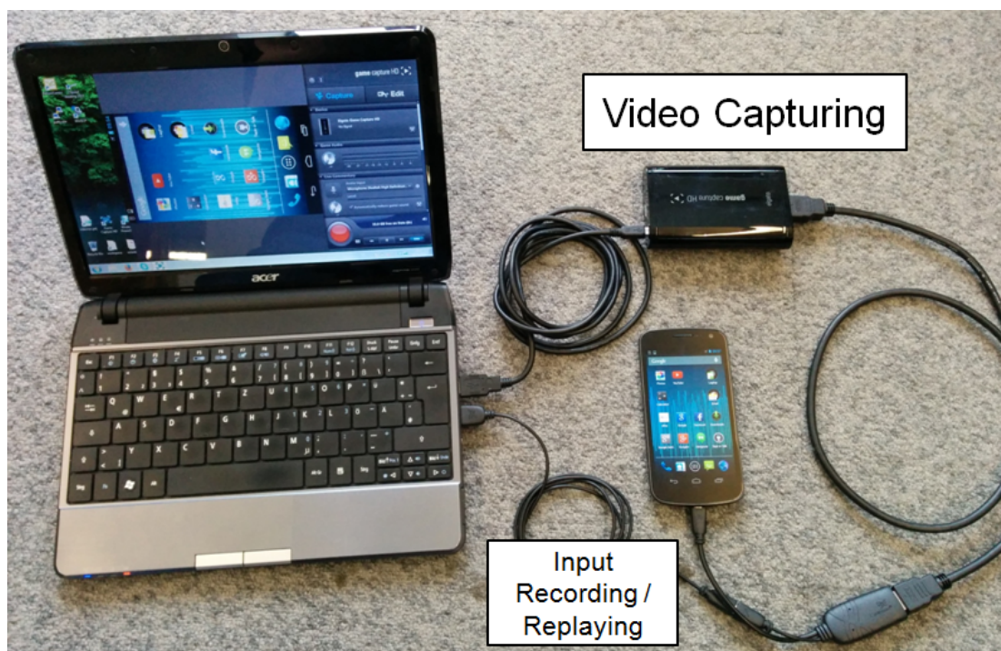
Figure 4.9: A video of the mobile screen output is captured by recording an HDMI signal with a video capture device like the Elgato Game Capture HD [178].
