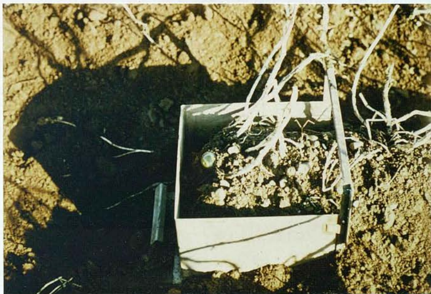
Fig. 29. Base plate forced horizontally into box.
