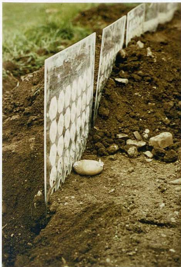
Fig. 23. Soil removed from non-planted side of Perspex template in preparation for sampling
