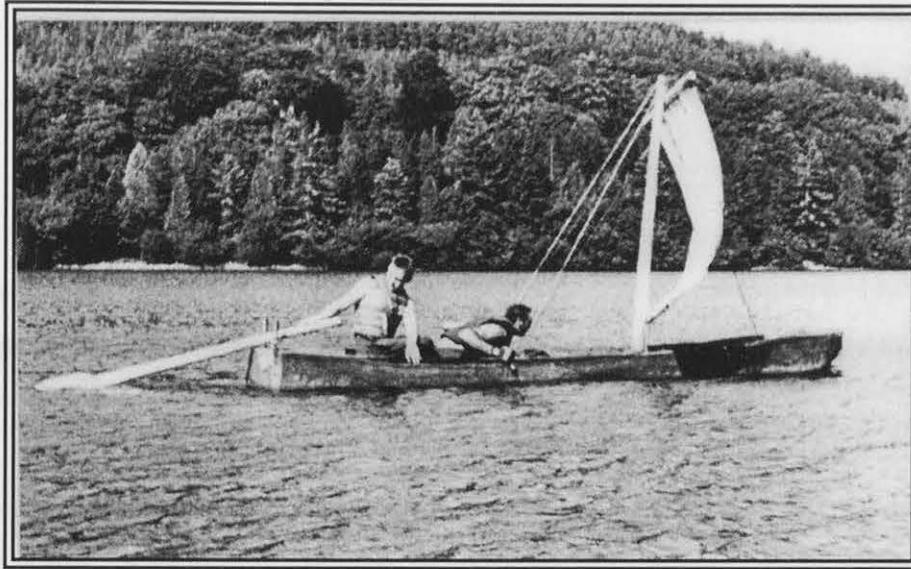
Plate 2.1: Daire, an experimental logboat, under sail without keel or leeboard.
