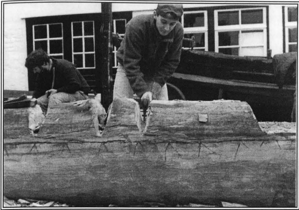
Plate 12.3: Removing excess external wood
