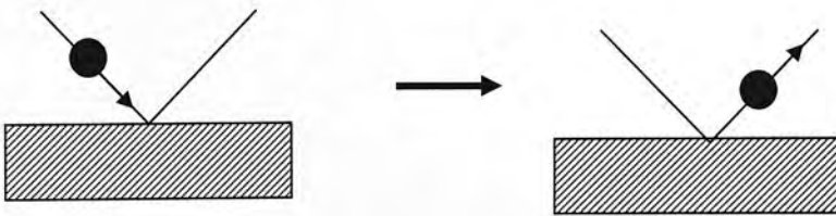
Figure 3.9b. Specular reflection collision at a solid node.
