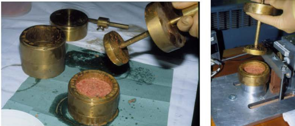
Figure 10. a) Compacted test sample b) transferred to shear tester.
