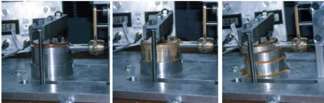
Figure 11. a) Axial load applied via hanger b) further fat extrusion after 5 minutes equilibration prior to shearing c) shearing complete.
