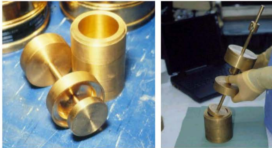
Figure 7. Proctor's impactor a) before and b) after modification
