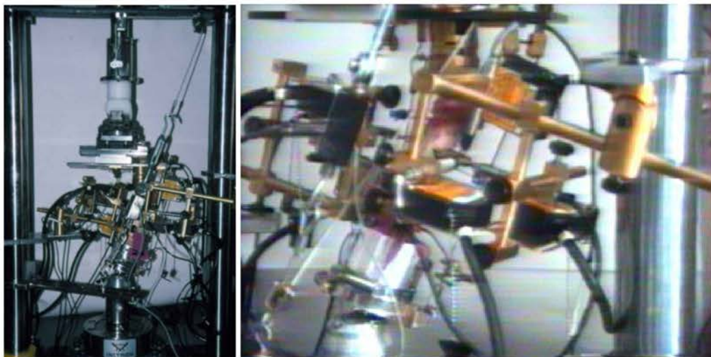
Figure 58. a) Instron set-up b) close-up of distal target orthogonal jig
