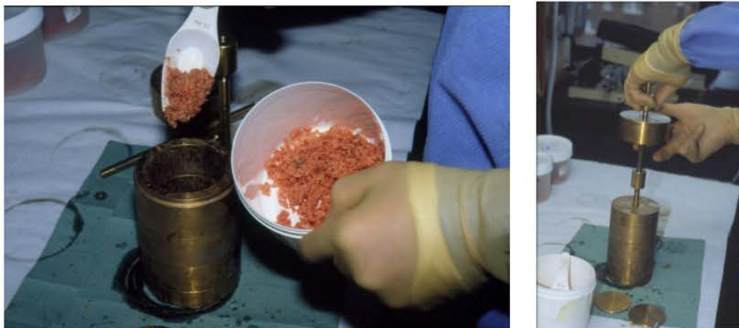
Figure 8. a) Test material introduced into impactor and b) compacted
