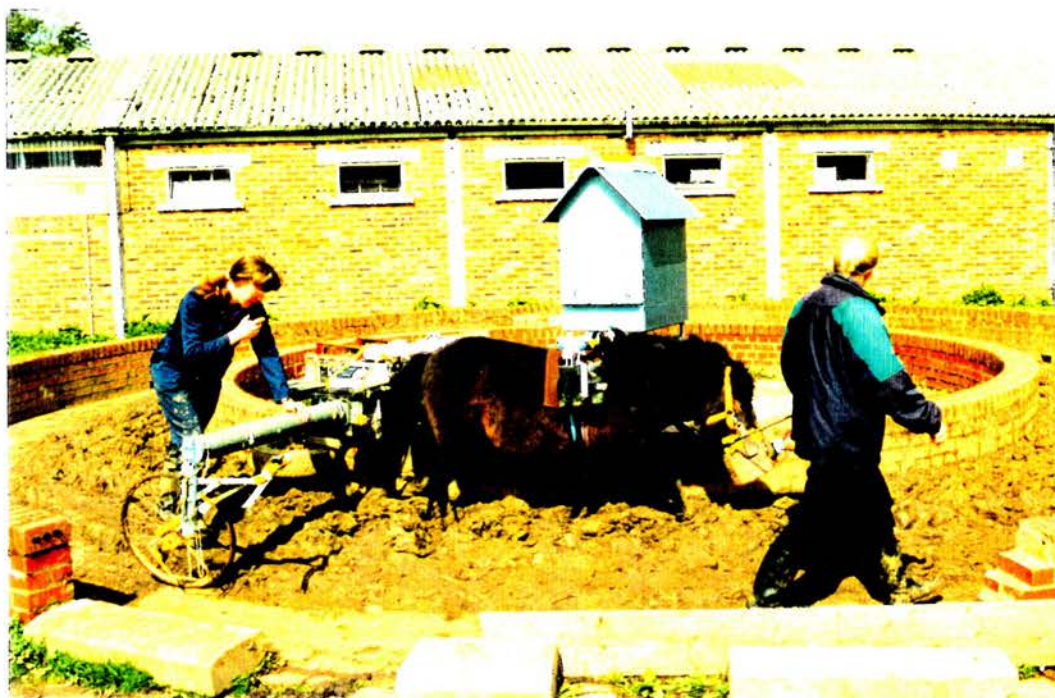
Plate 2.2; A Shetland pony being led round the mud-filled circular race whilst carrying an Oxylog and wearing a closed face-mask. The data viewer and distance wheel were secured to the draught bar which was pushed by a second person who also recorded data using a dictaphone.
