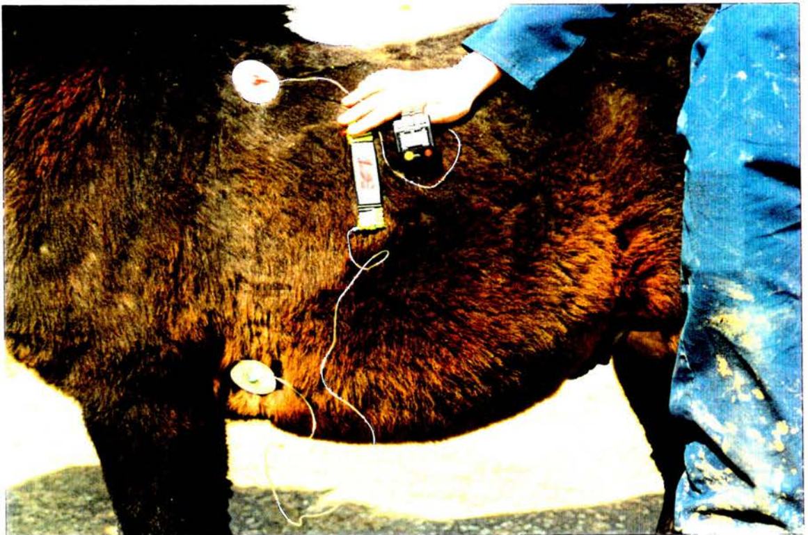
Plate 2.5; A Polar-Electro heart rate monitor in position on a Shetland pony. The ECG electrodes (white discs) were wired to the transmitter which emitted signals recorded by the watch-receiver.
