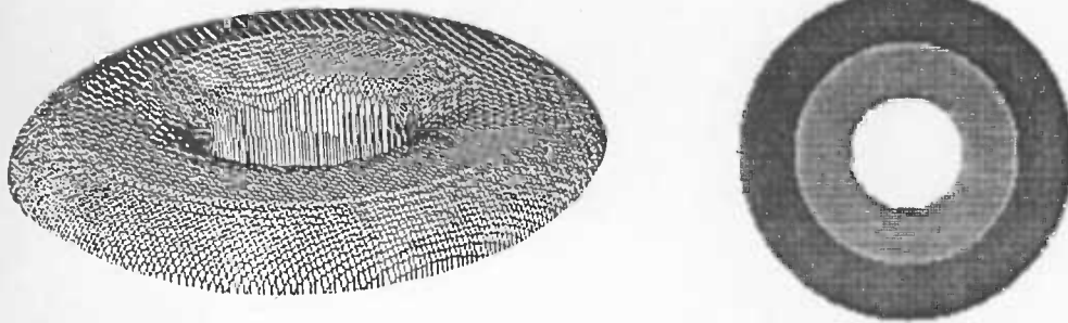
Figure 5.3.2. Segmentation of a torus (synthetic data) using only the KH sign images resulting from scale space smoothing (scale t = 6 ).
