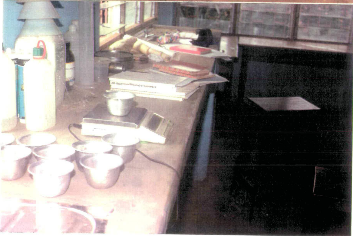
Plate 2.2: Volumetric water, air and solid content and air:water ratio determination of the rooting media used in the media experiments.
