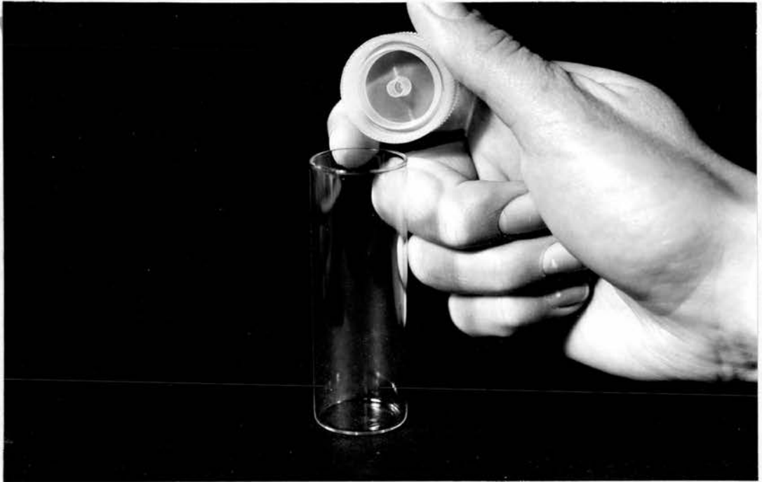
1a) 1" x 3" 'Samco' tube with clear plastic lid from 'Sterilin' disposable universal container
